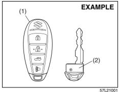
Your vehicle comes with two identical keyless start system remote controllers (1), each with a detachable key (2) housed inside.
